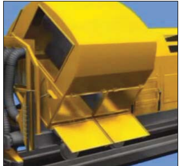
Side emptying action by tilting the container Disadvantage: emptying at only one place
