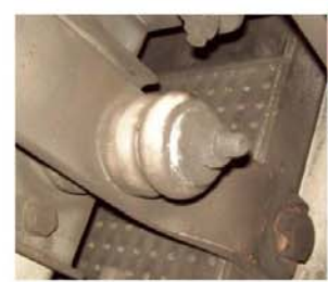
Figure H Not on Layout Durasteel 0.25m 2 Undercarriage, Above air exhaust system next to resistor grids Amosite & Chrysotile
