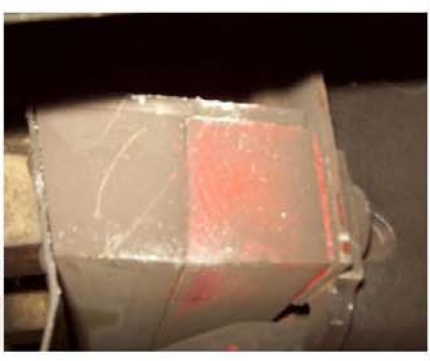
Figure E 2no. <1m 2 Cement Panel To switch behind large arc chutes Chrysotile
