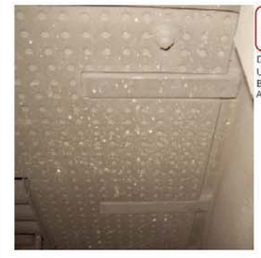
Figure K Durasteel 0.25m 2 Undercarriage Between wheels Amosite & Chrysotile
