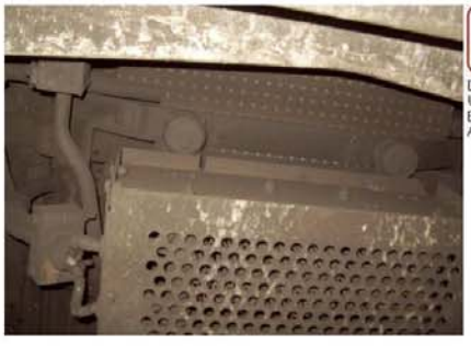
Figure I Not on Layout Durasteel 0.25m 2 Undercarriage, Between wheels Amosite & Chrysotile
