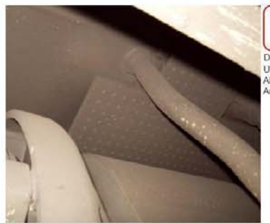
Figure H Not on Layout Durasteel 0.25m 2 Undercarriage, Above air exhaust system next to resistor grids Amosite & Chrysotile
