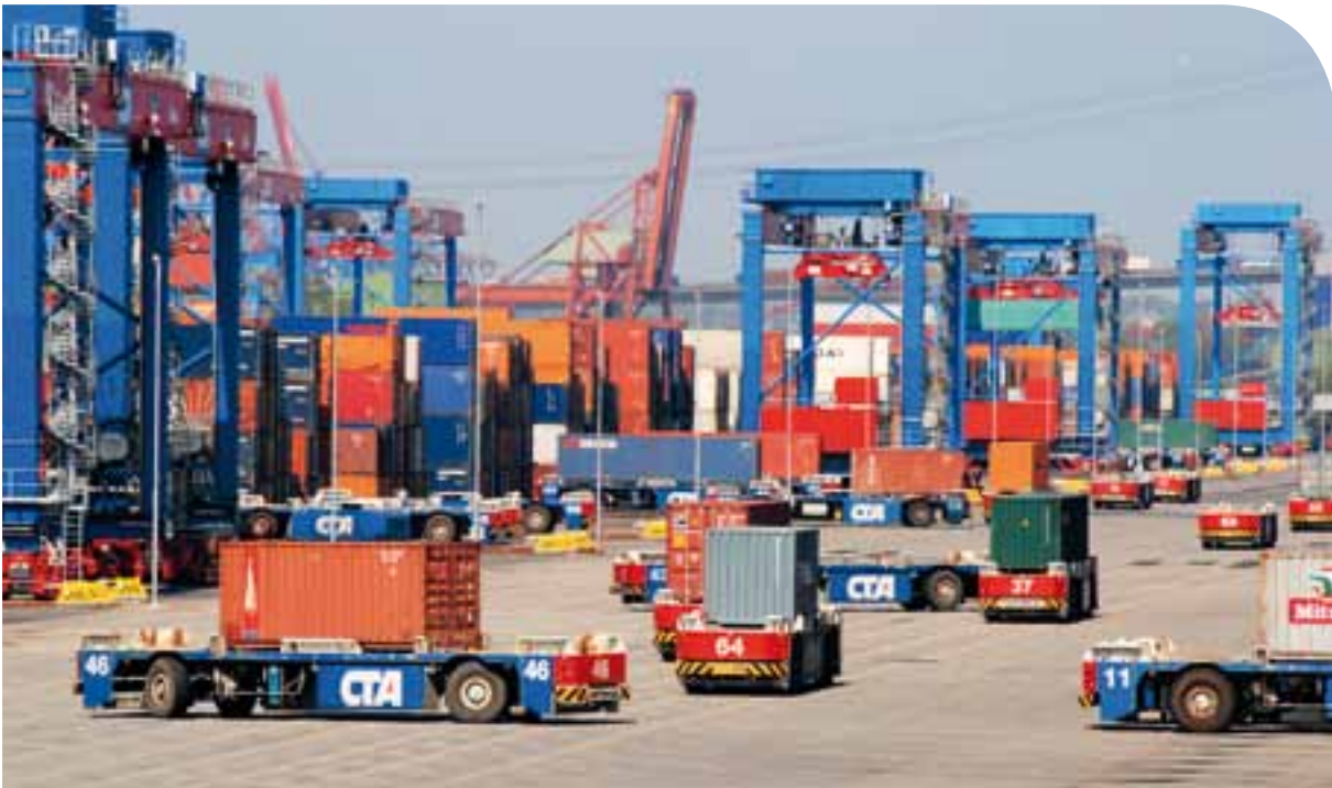
Automatic Guided Vehicles (AGVs) help to reduce emissions, especially if they have an electric drive.
