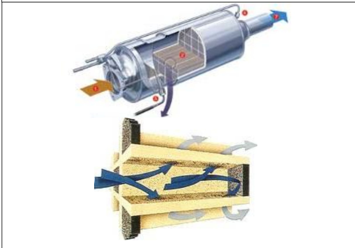
Figure 3.1: An illustration of a Diesel Particulate Filter
