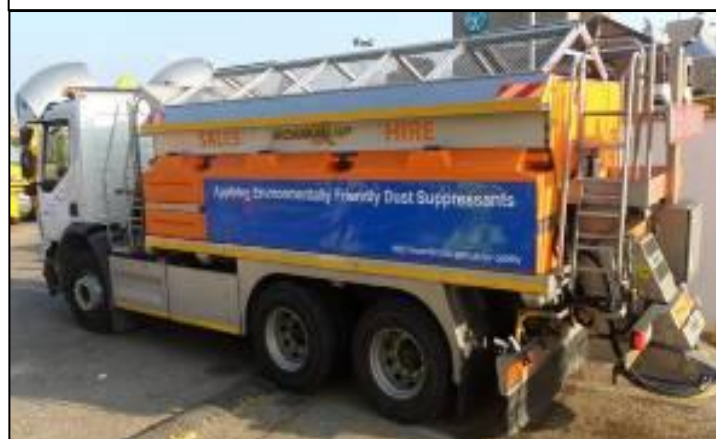
Figure 6.2: Winter Servicing Vehicle fitted to Apply Dust Suppressants
