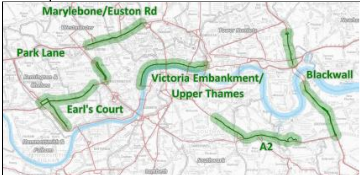
Figure 6.2: 6 Road corridors (covering 20 miles) that received regular applications of CMA as part of the CAF trial
