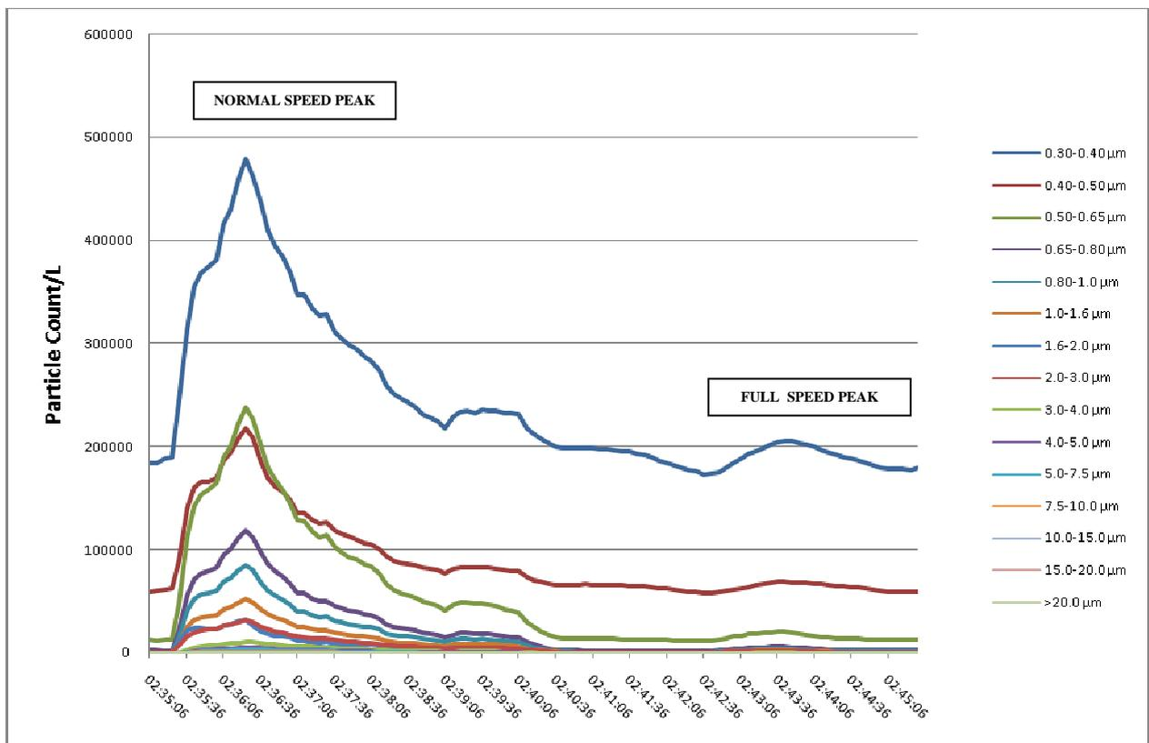
Figure 17. Particle count data for test in cess in tunnel between Moorgate and Barbican Stations
