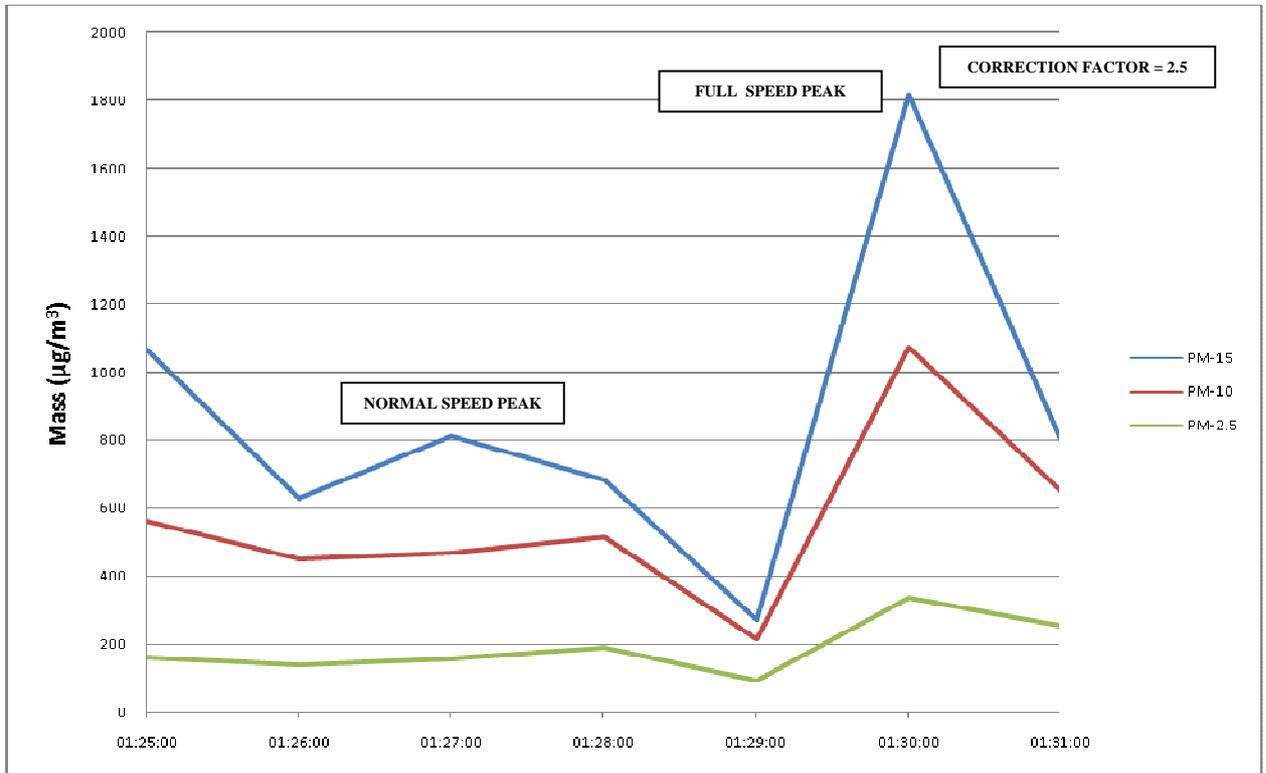
Figure 25. Particle count data for test in 6 foot at east end of Euston Square Station
