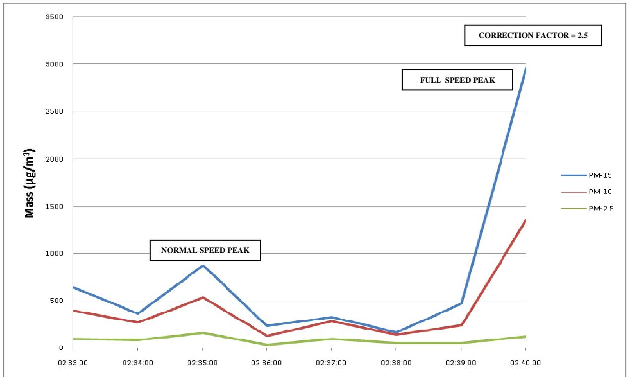
Figure 29. Particle count data for test in cess area in tunnel between King’s Cross and Farringdon Stations
