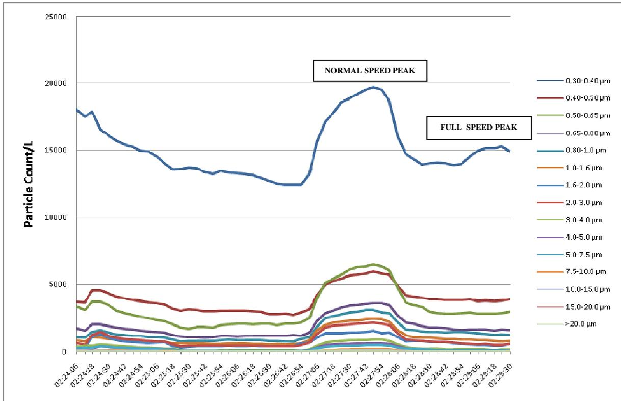
Figure 38. Particle mass data for test in cess area in tunnel between Aldgate and Liverpool Street Stations
