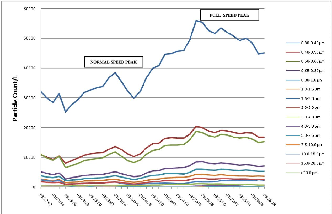
Figure 30. Particle mass data for test in cess area in tunnel between King’s Cross and Farringdon Stations
