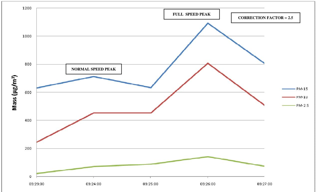
Figure 31. Particle count data for test in cess area of open section between King's Cross and Farringdon Stations
