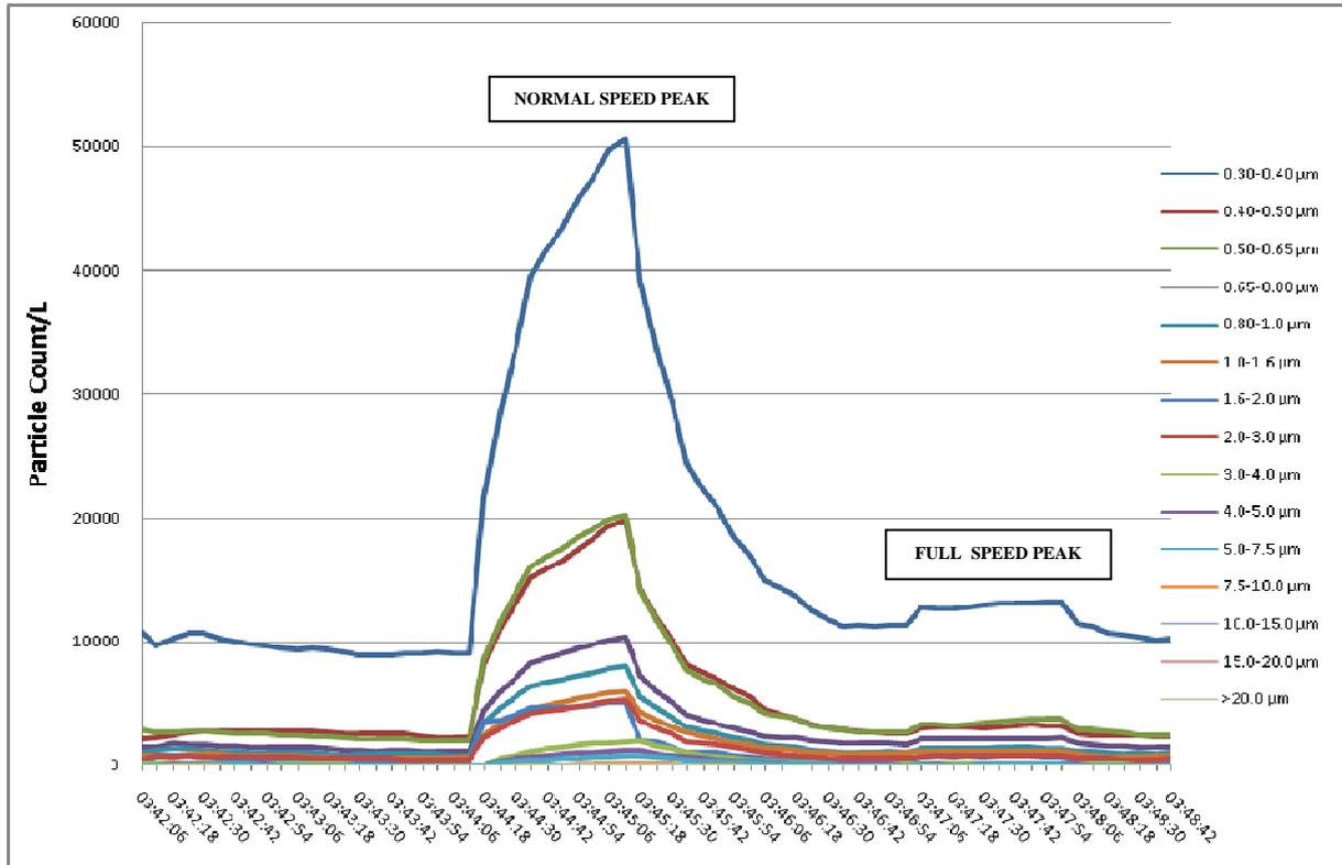
Figure 44. Particle mass data for test in cess area in tunnel between Liverpool Street and Moorgate Stations
