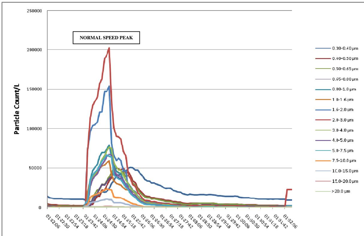
Figure 34. Particle mass data for test in cess at east end of platform at Aldgate Station
