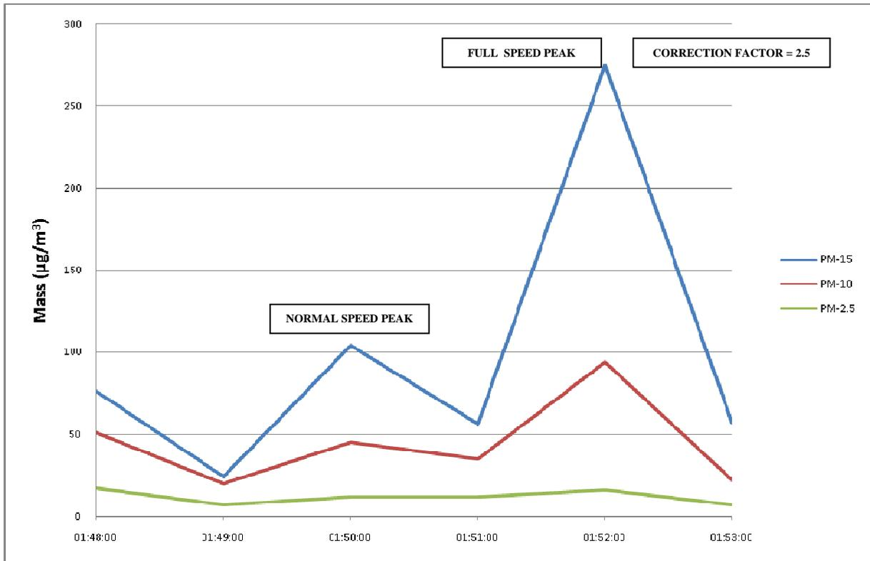
Figure 37. Particle count data for test in cess area in tunnel between Aldgate and Liverpool Street Stations
