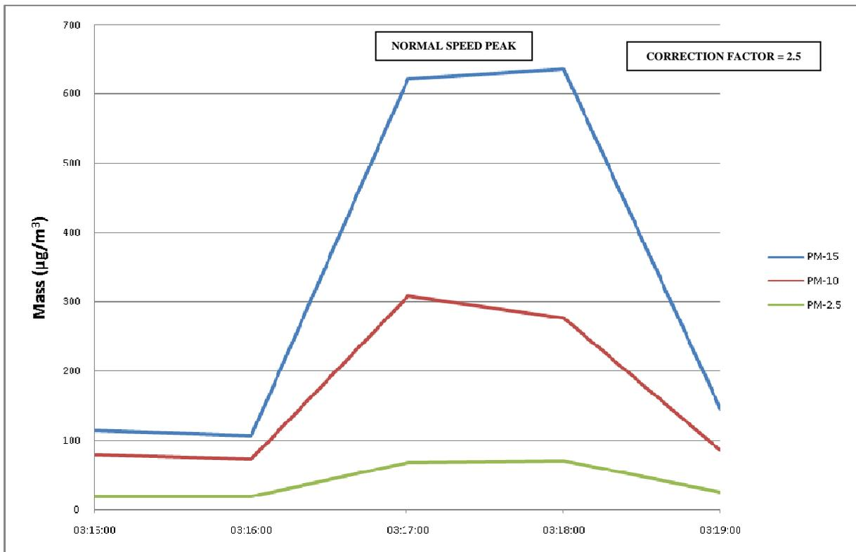
Figure 43. Particle count data for test in cess area in tunnel between Liverpool Street and Moorgate Stations
