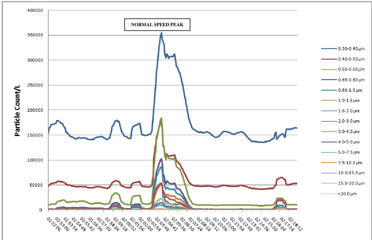
Figure 16. Particle count data for test in cess at west end of Moorgate Station
