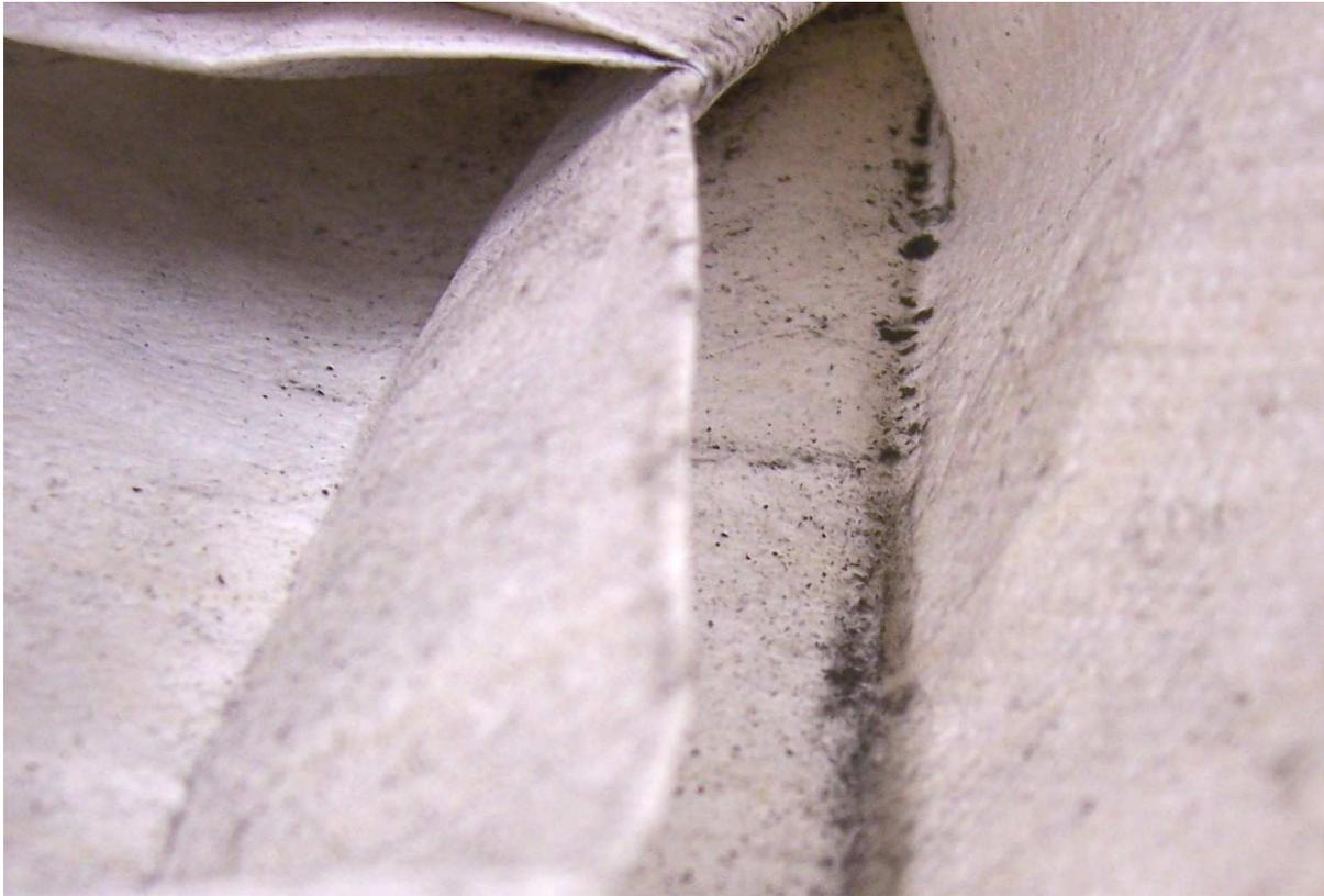
**Figure 11. Dust collected in vacuum bag from test at King’s Cross Station**
