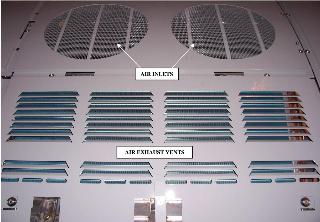
Figure 4. View from underside of S Stock brake fan exhaust showing baffle plate
