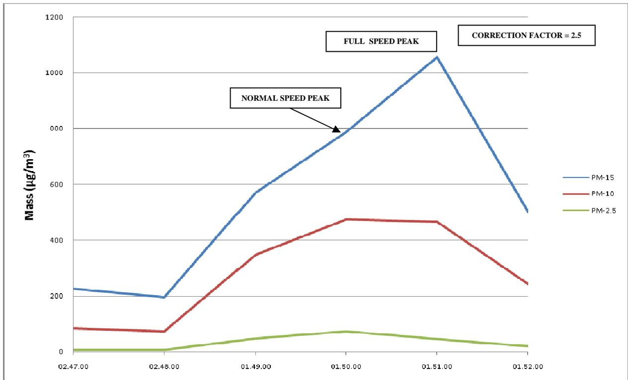
Figure 21. Particle mass data for test in cess at west end of platform at Great Portland Street Station
