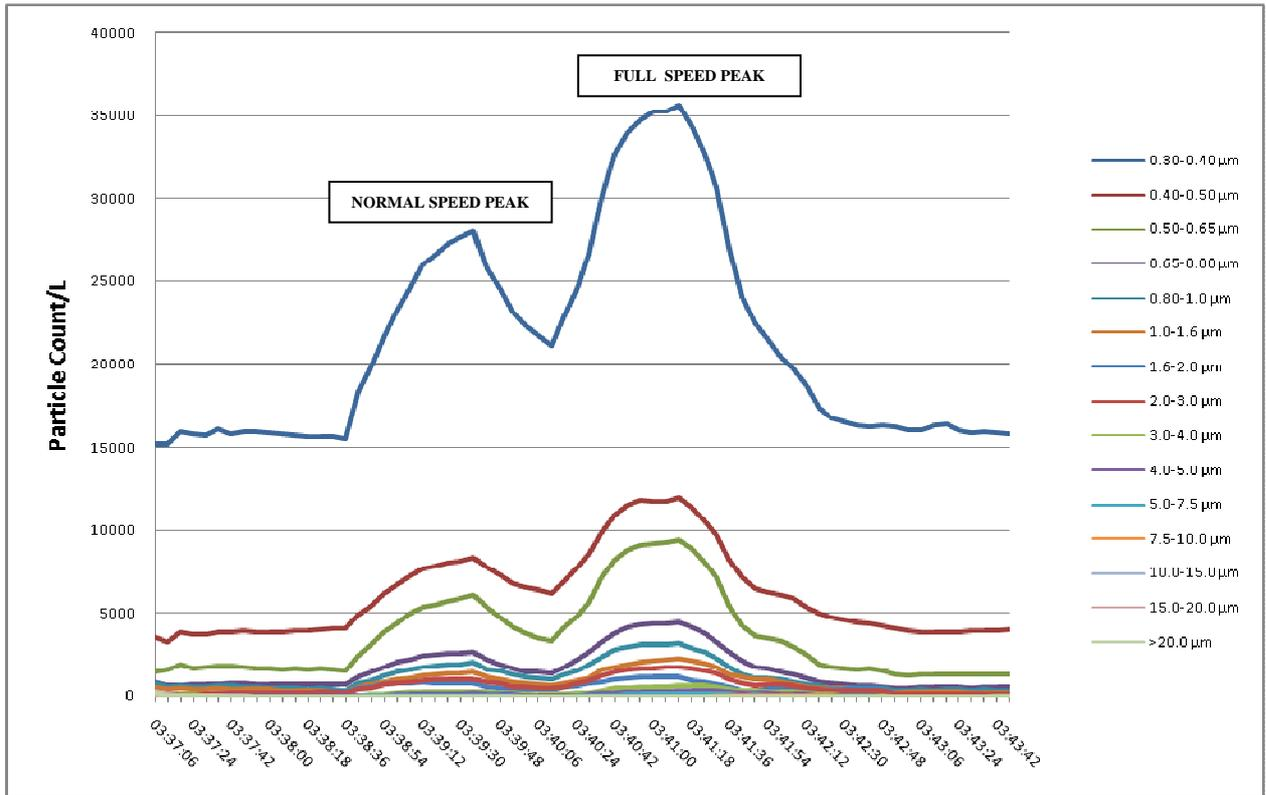
Figure 32. Particle mass data for test in cess area of open section between King's Cross and Farringdon Stations
