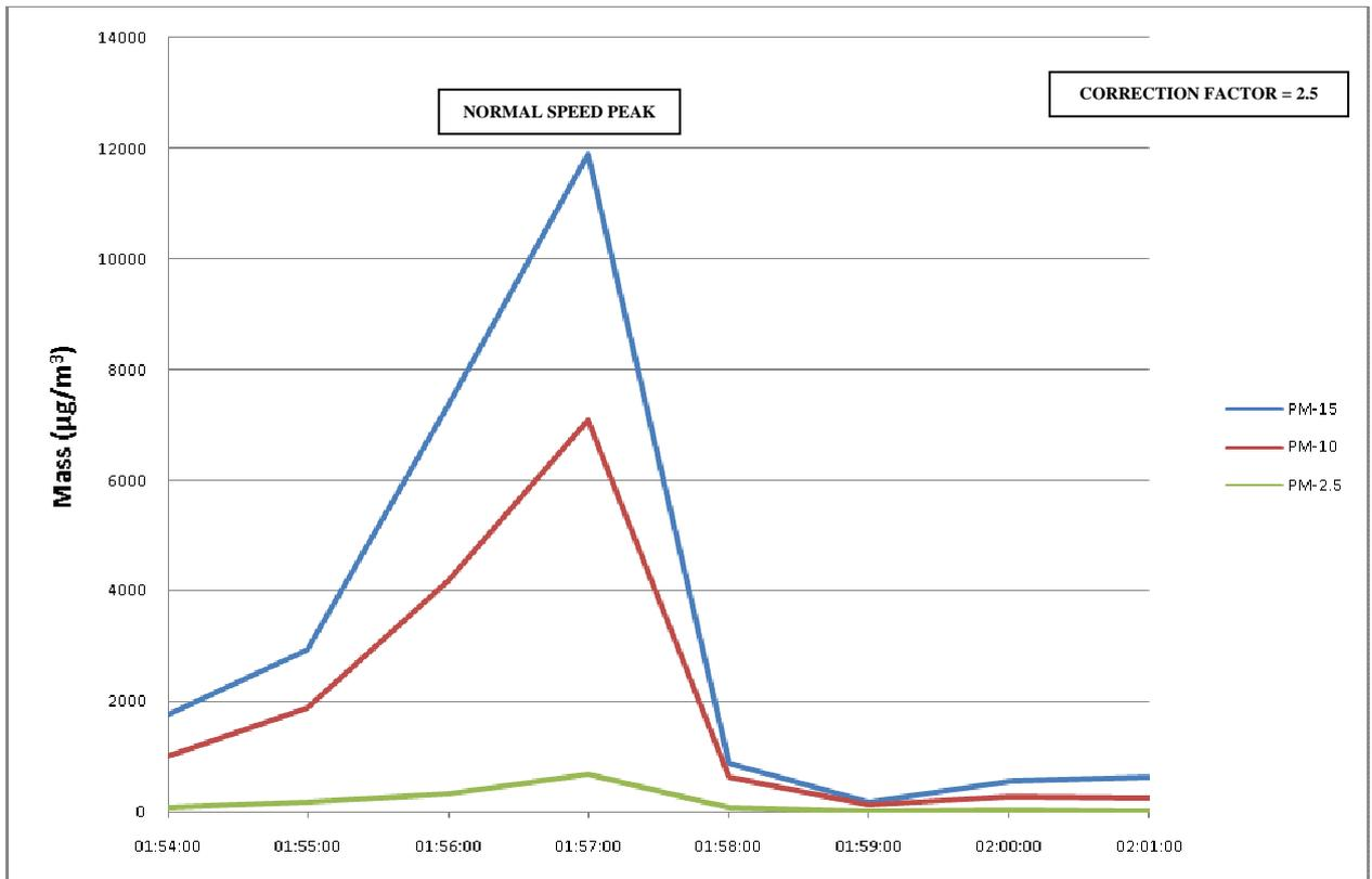
Figure 19. Particle mass data for test in 6 foot in tunnel 200m north of Baker Street Station
