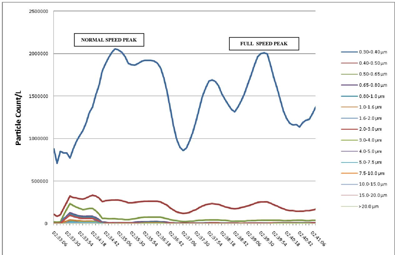
Figure 28. Particle mass data for test in cess area at east end of platform at King's Cross Station
