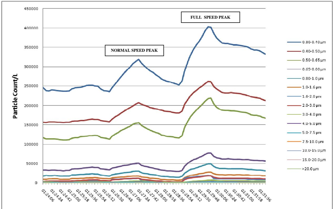
Figure 24. Particle mass data for test in cess at west end of platform at Euston Square Station
