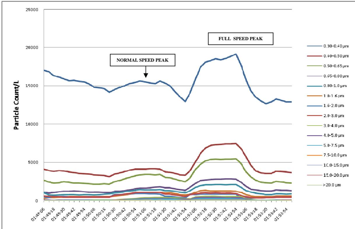
Figure 36. Particle mass data for test in 6 foot at west end of platform at Aldgate Station
