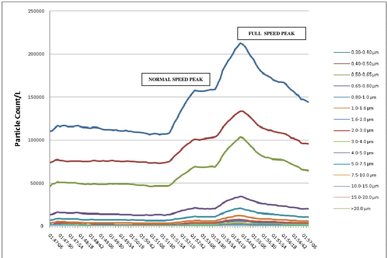
Figure 26. Particle mass data for test in 6 foot at east end of Euston Square Station
