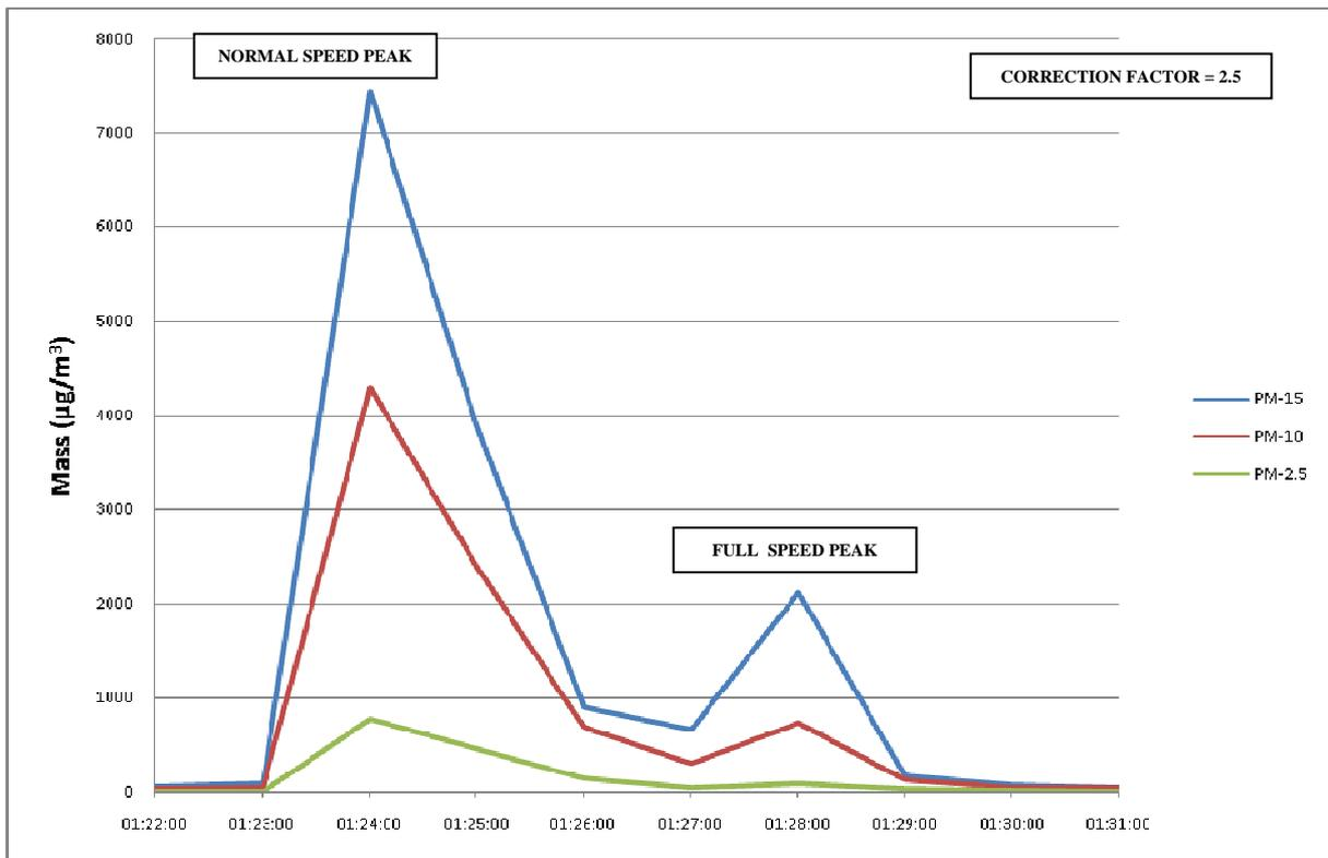
Figure 35. Particle count data for test in 6 foot at west end of platform at Aldgate Station
