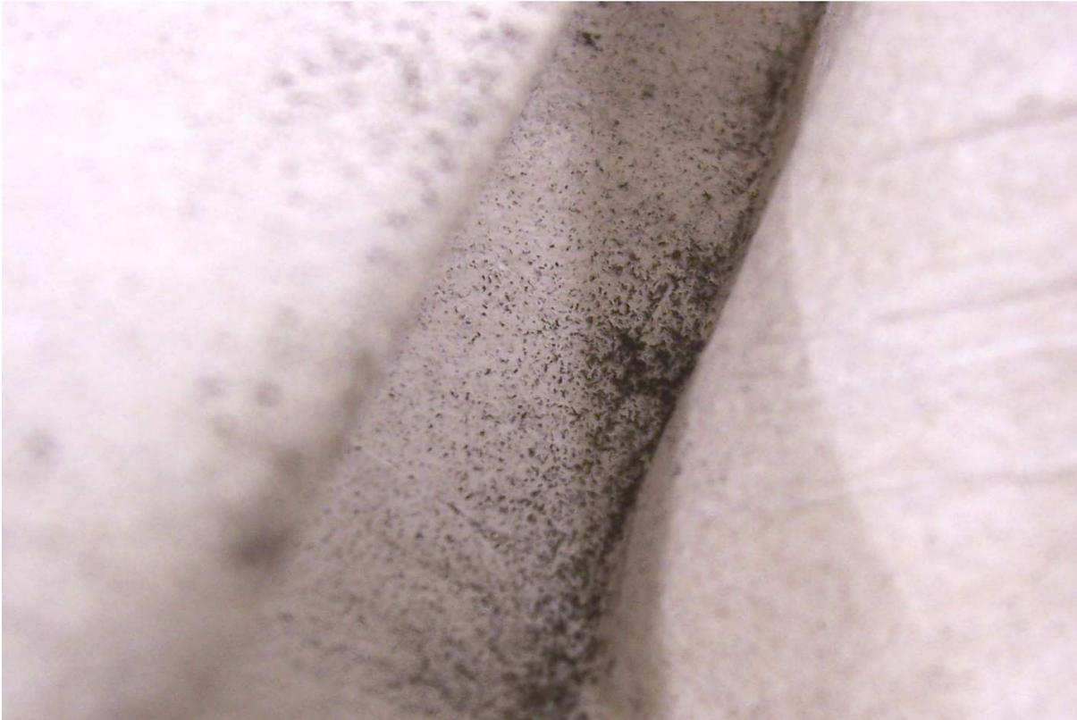
**Figure 12. Dust containing gritty particles collected from test in tunnel between King’s Cross and Farringdon Stations**
