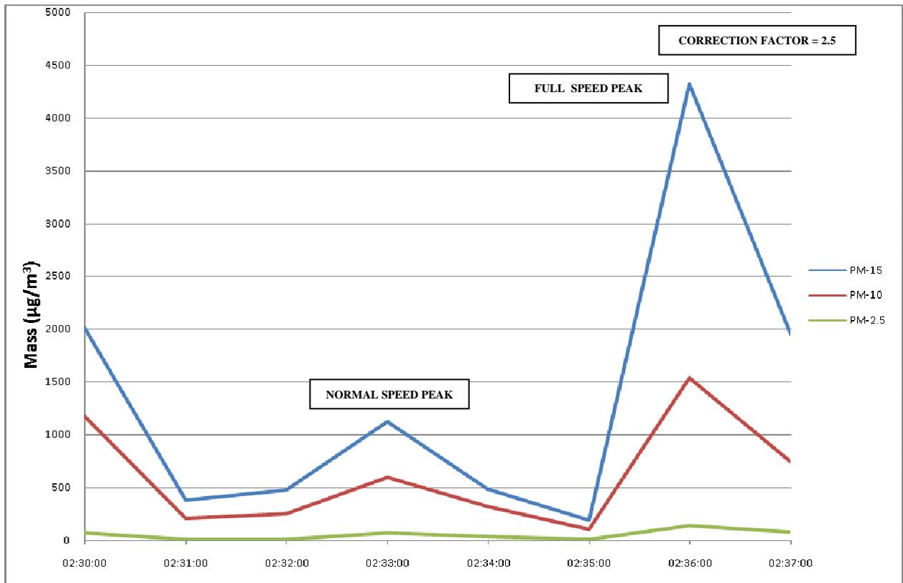
Figure 20. Particle mass data for test in cess in tunnel 200m north of Baker Street Station
