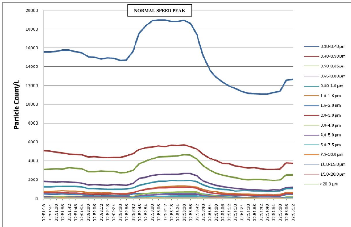
Figure 40. Particle mass data for test in cess area at east end of platform at Liverpool Street Station
