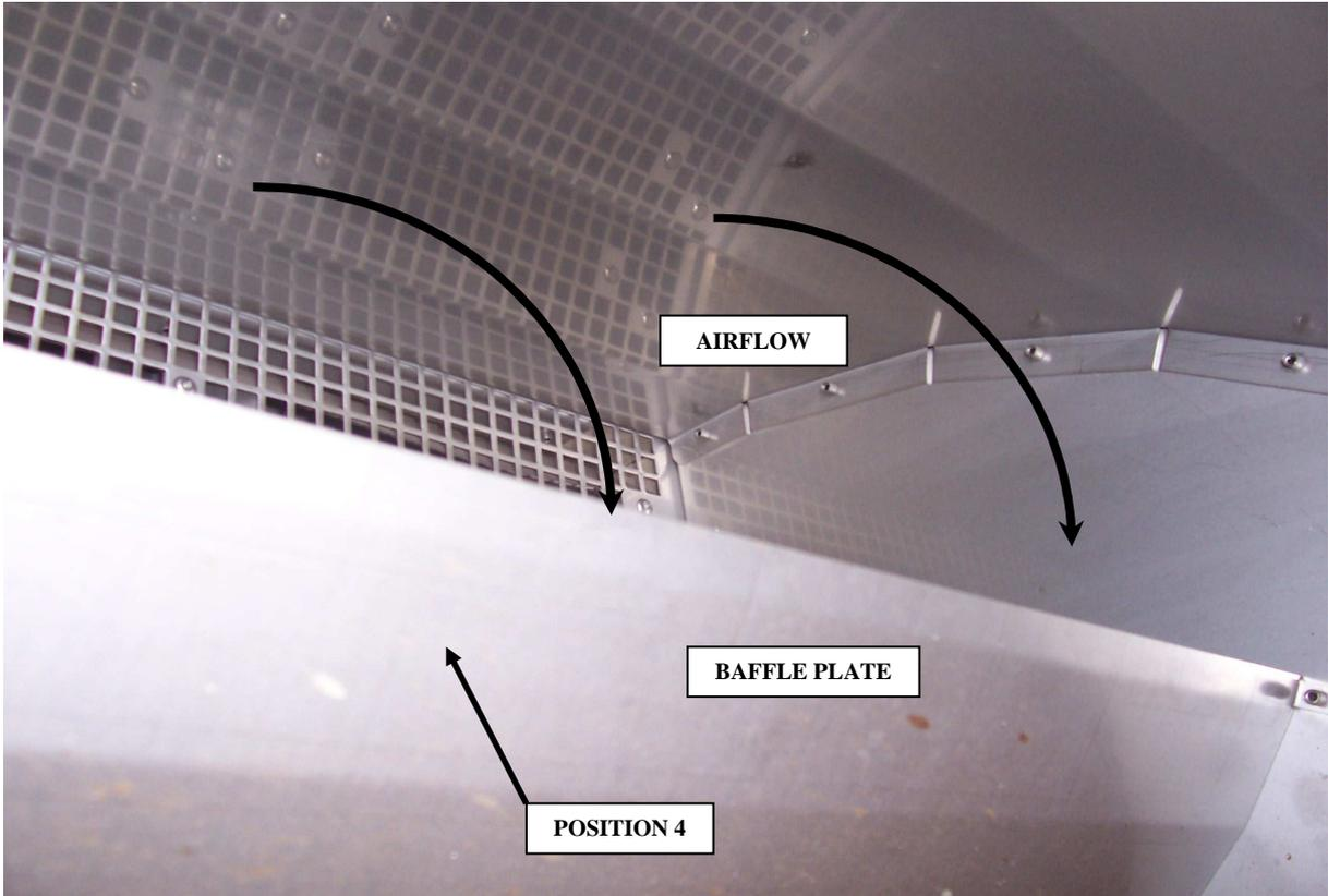
Figure 5. Underside view of small directional vent behind main exhaust of brake fan
