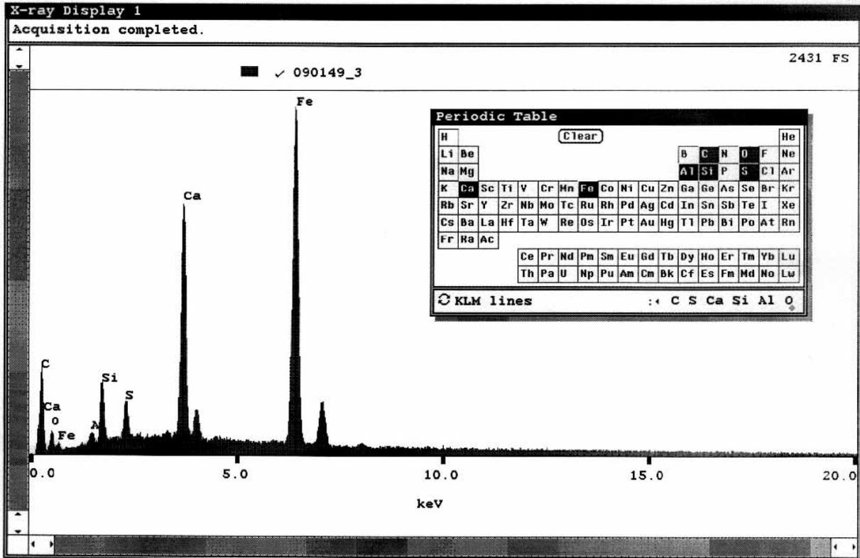
Figure 48. X-ray spectrum of dust from ballast collected in cess area at Aldgate Station
