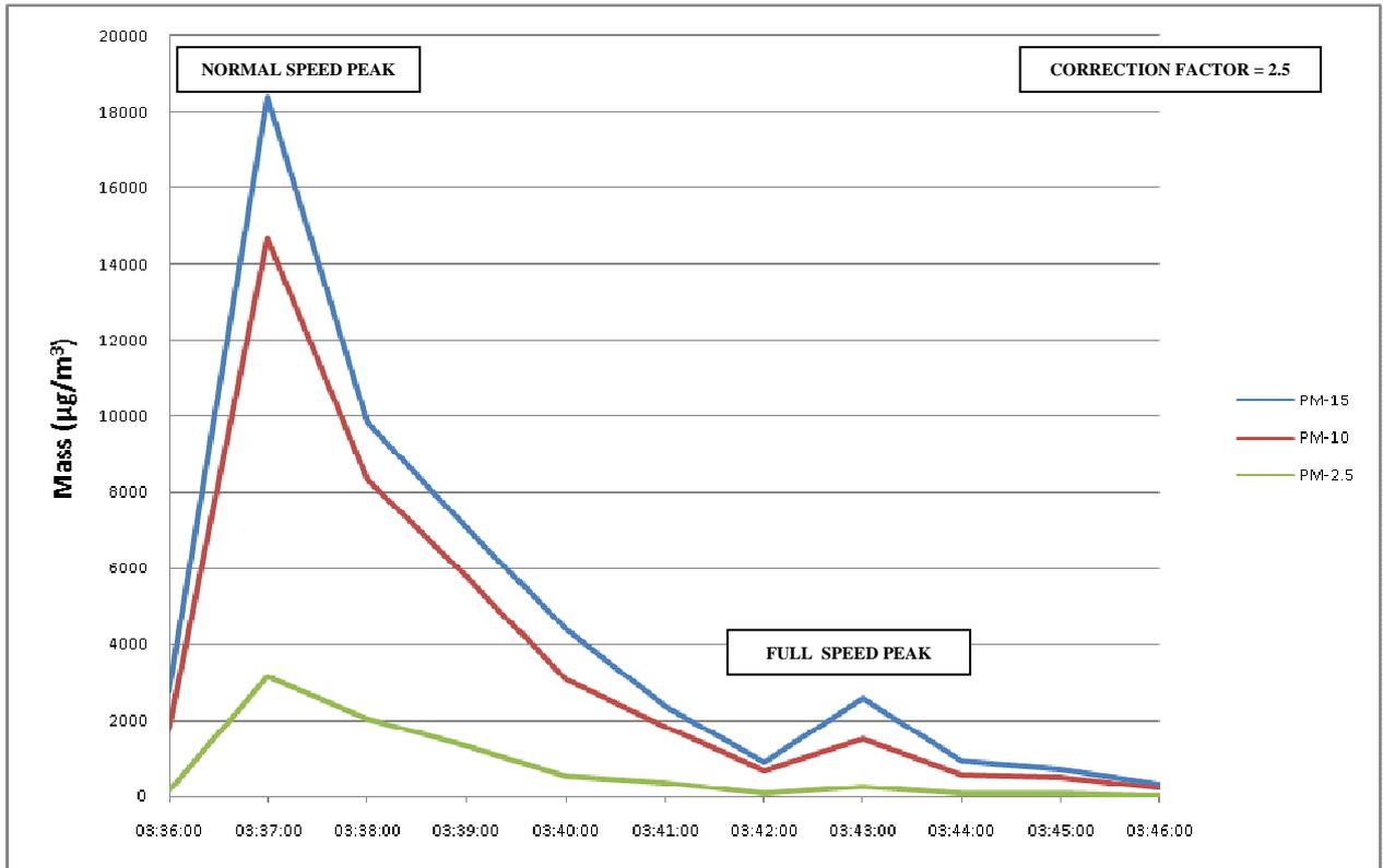
Figure 22. Particle mass data for test in 6 foot area at east end of platform at Great Portland Street Station
