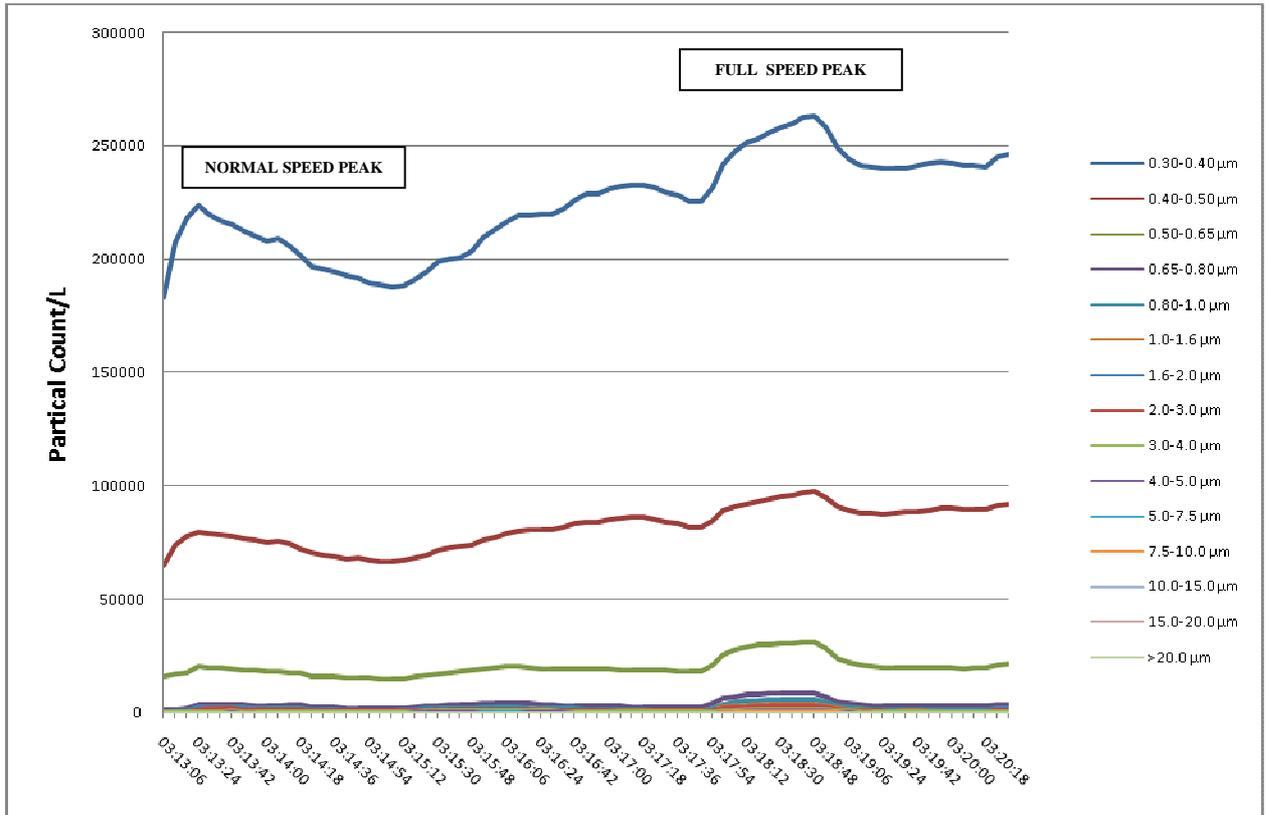
Figure 18. Particle mass data for test in cess at Baker Street Station platform 4
