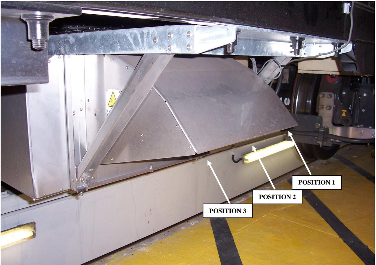
Figure 3. Top view of air inlets and exhausts of S Stock train HVAC unit
