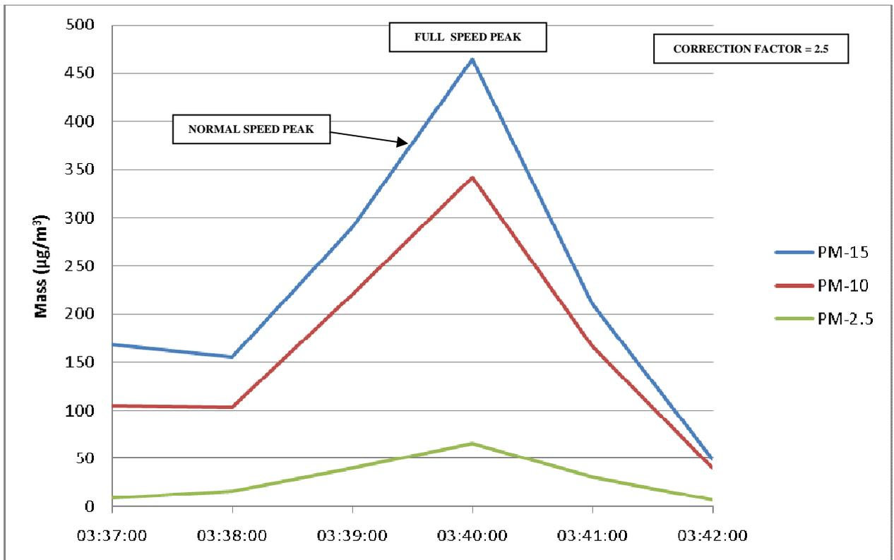
Figure 33. Particle count data for test in cess area at east end of platform at Aldgate Station
