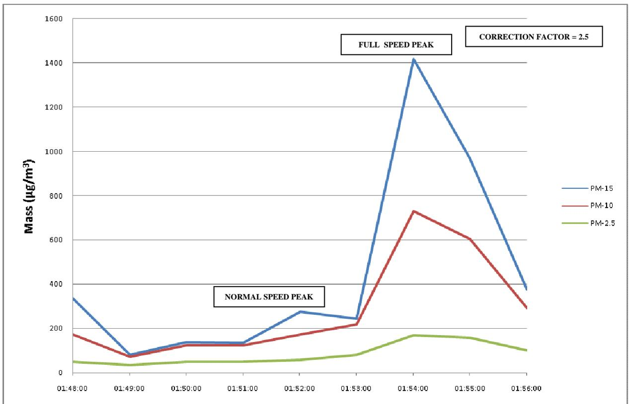
Figure 27. Particle count data for test in cess area at east end of platform at King's Cross Station
