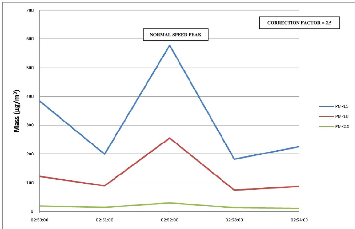
Figure 41. Particle count data for test in cess area at west end of platform at Liverpool Street Station
