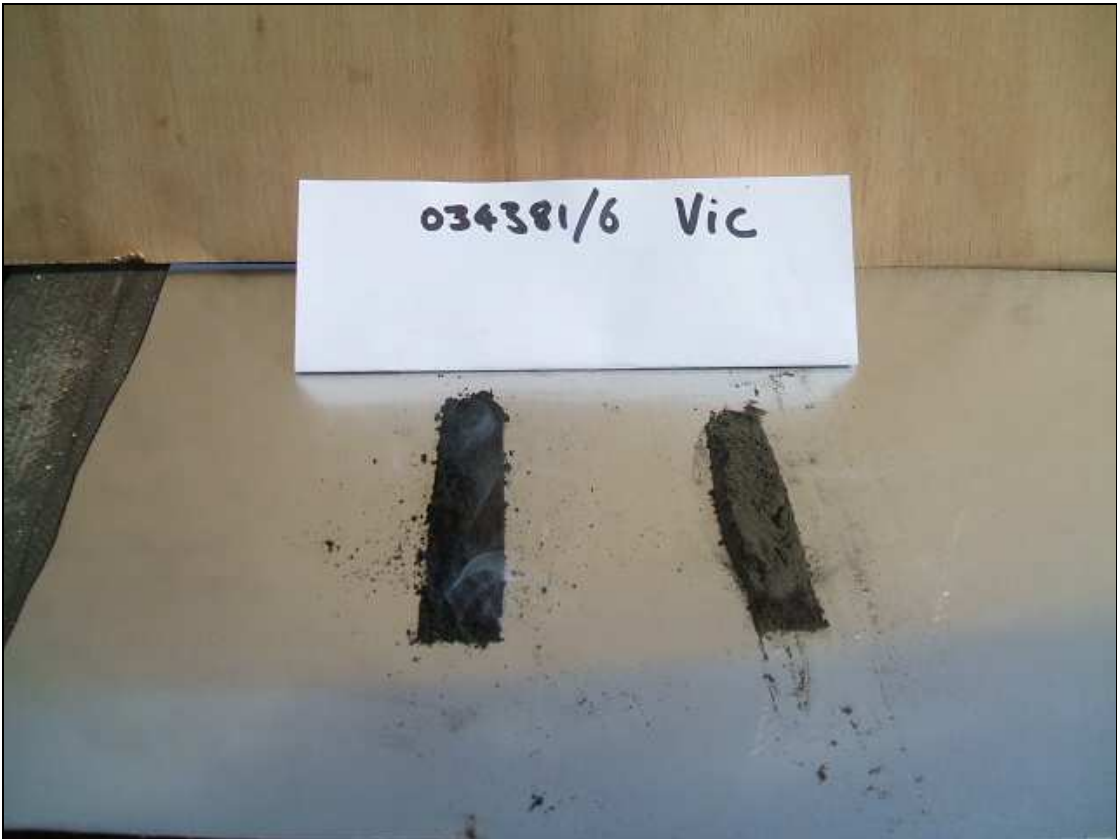
Figure 4: Qualitative ignition test of dust samples
