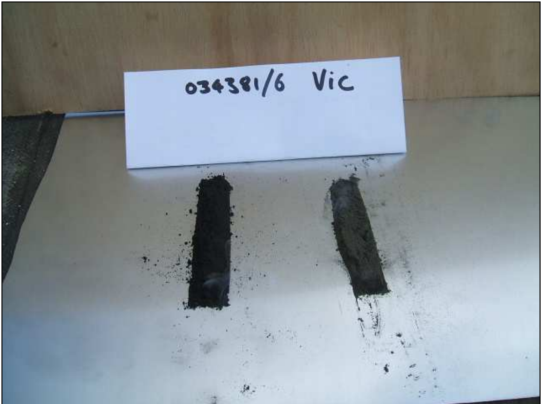
Figure 4: Qualitative ignition test of dust samples
