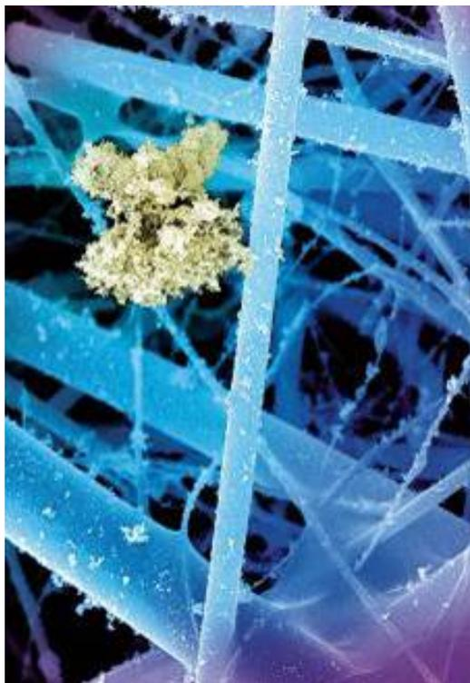
Photo of soot particles in air filter
