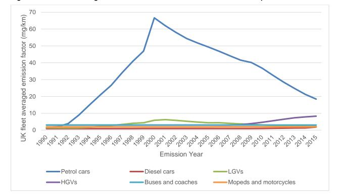
Figure 3-6 UK fleet averaged NH<sub>3</sub> hot exhaust emission factors for road transport
