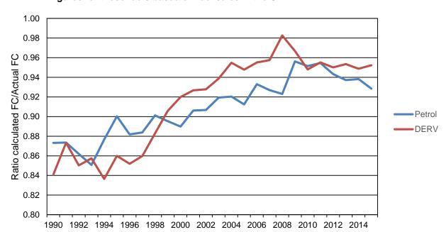
Figure 3-1 Ratio of calculated consumption of petrol and diesel fuel based on traffic movement and fuel consumption factors summed for different vehicle types to the DUKES figures for these fuels based on fuel sales in the UK.
