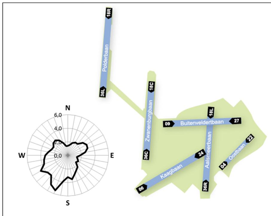
Fig. 2. The six runways, including flight codes and the wind rose (%) in 2012 at Schiphol.
