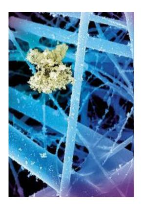
Photo of soot particles in air filter
